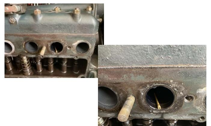
I separated the carburetor and the main jet did break off and found its way into the number one intake port. I next removed the head to check the number one intake valve but did not notice any damage.
