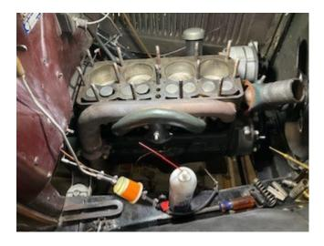
Next I removed the intake and exhaust manifolds. Well much to my horror was the main carburetor jet lying in the block intake port.
